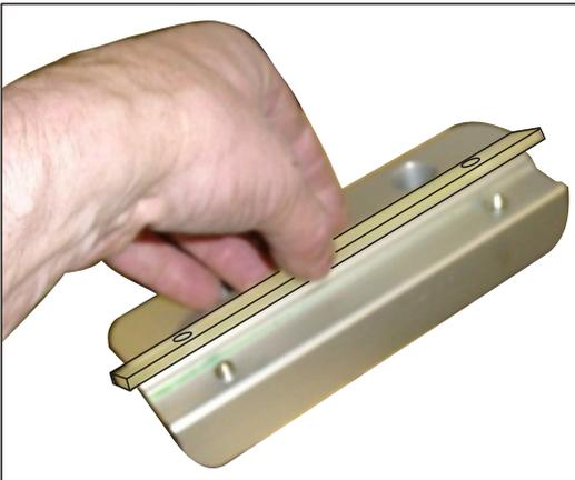
5. Mount the clamp with screw, washer and nut.
