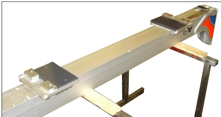
7. The bolster is now ready to be turned the right way up, and placed on the chassis. Plastic plates will be used for both clamp and friction attachment.
