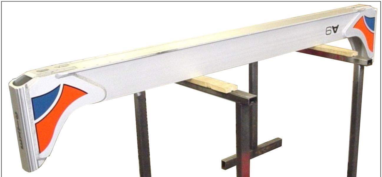
2. Measure the width on the outside of the chassis frame and add 6 mm (0.23 inches). Example: If the frame width is 1250 mm (49.2 Inches), the distance between the attachment framestops must be 1256 mm (49.4 inches). Use the mark in the middle of the bolster to get a correct measurement.
